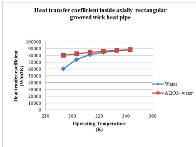
Graph 5: Heat transfer coefficient inside axial rectangular grooved wick heat pipe
