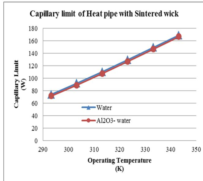
Graph 4: Capillary limit of sintered wick heat pipe
