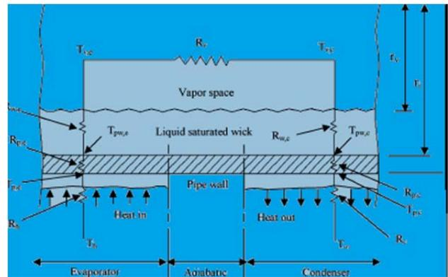
**Fig. 4: Internal Resistance approach and parameters**
