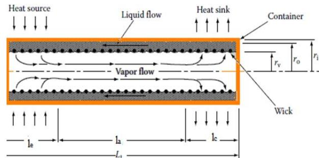
Fig. 2: Schematic representation of the Horizontal heat pipe
