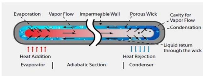
Fig. 1: Working of the Horizontal heat pipe
