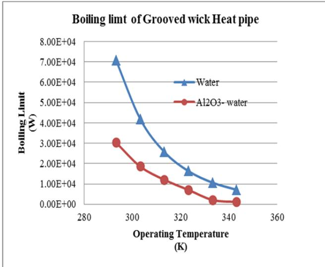
Graph 1: Boiling limit of grooved wick Heat pipe
